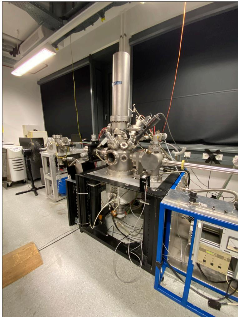
**Figure 4** Photo of a time-of-flight mass spectrometry in a nuclear chemical laboratory (TOF-MS). Source: Christiane Schürkmann.
